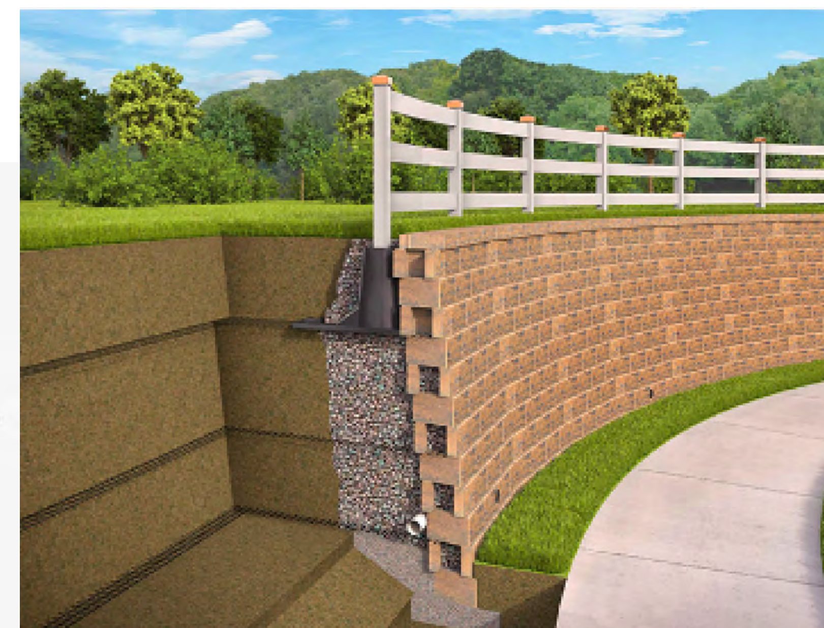
2 FENCE POST INSTALLATION USING SLEEVE-IT RW-6 SCALE: 1/2" = 1'
