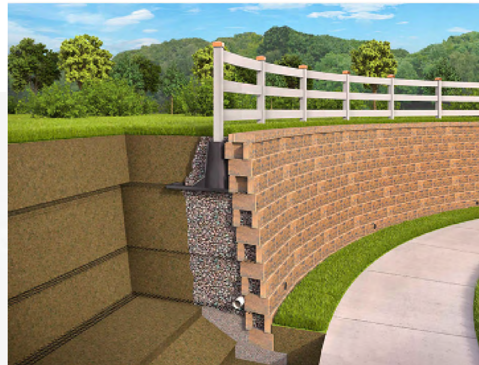
2 FENCE POST INSTALLATION USING SLEEVE-IT RW-6 SCALE: 1/2" = 1'
