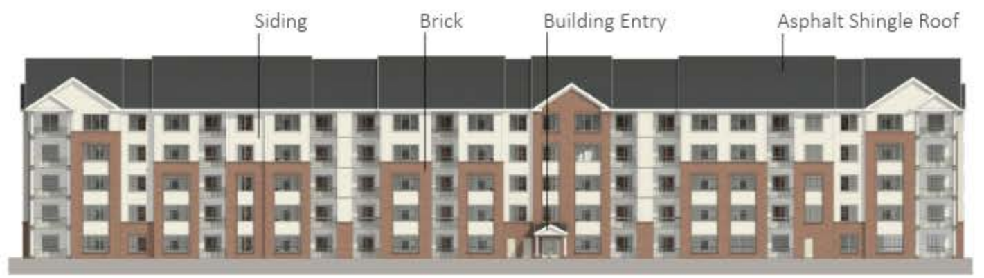
Typ 5-ST Building South Elevation
