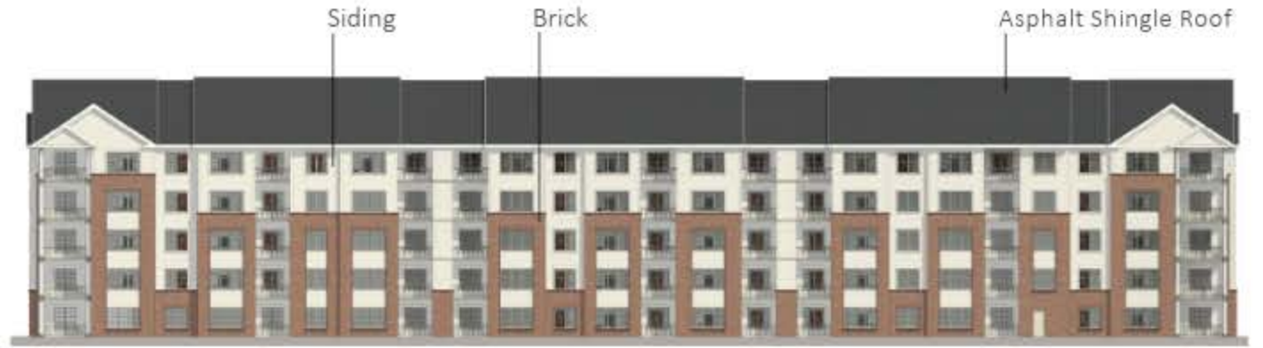
Typ 5-ST Building North Elevation
