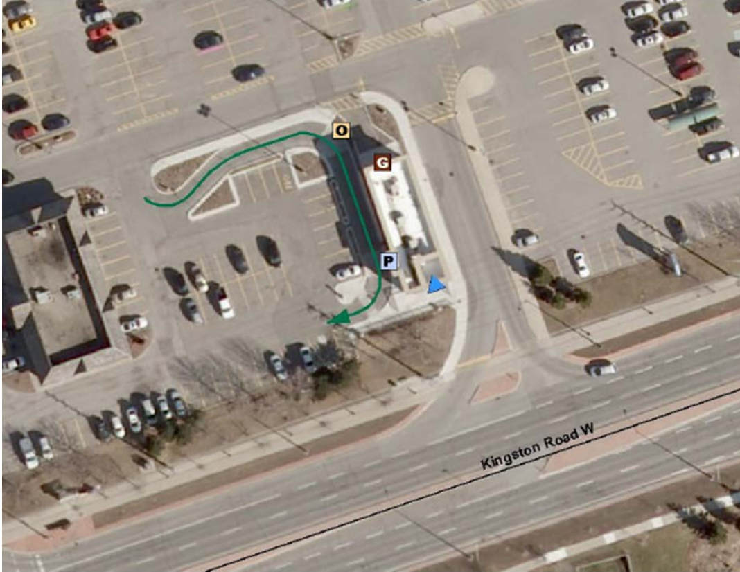
Example site layout: Coffee Shop Site in Ajax, Ontario (Queuing/Stacking Lane is in Green)
