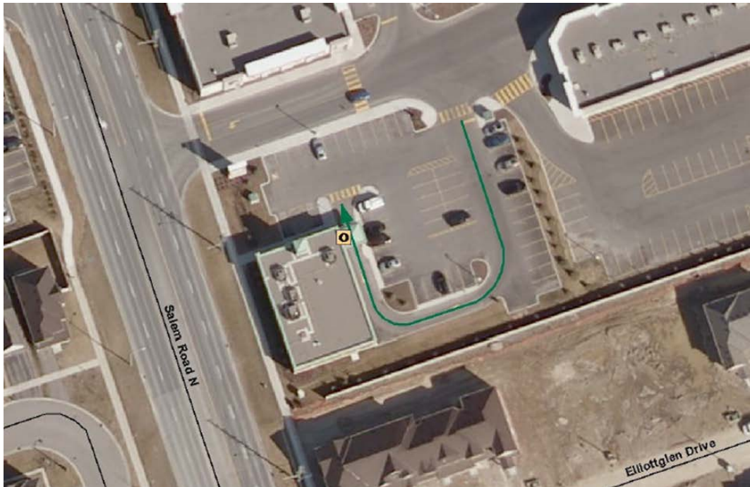
Example site layout: Bank Site in Ajax, Ontario (Queuing/Stacking Lane is in Green)
