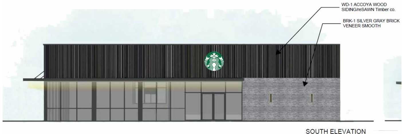
Exhibit #36: Starbucks Building Elevations
